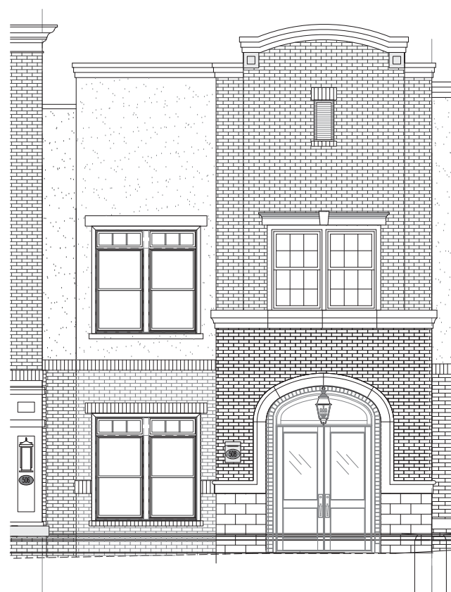
3 A5.3 ELLISON UNIT 106 NORTH EXTERIOR ELEVATION SCALE: 1/4" = 1'-0"
