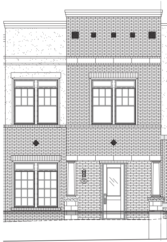
1 A5.4 ELLISON UNIT 108 NORTH EXTERIOR ELEVATION SCALE: 1/4" = 1'-0"
