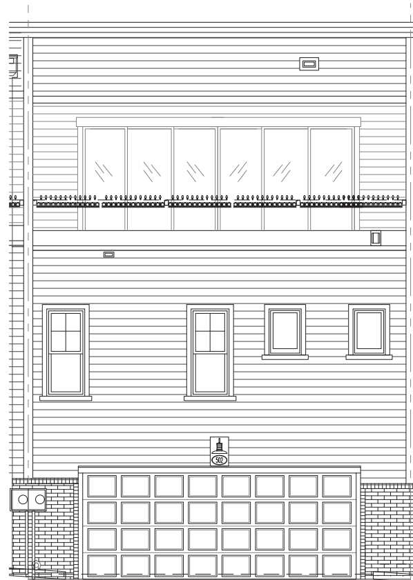
1 A5.4 ELLISON UNIT 108 SOUTH EXTERIOR ELEVATION SCALE: 1/4" = 1'-0"
